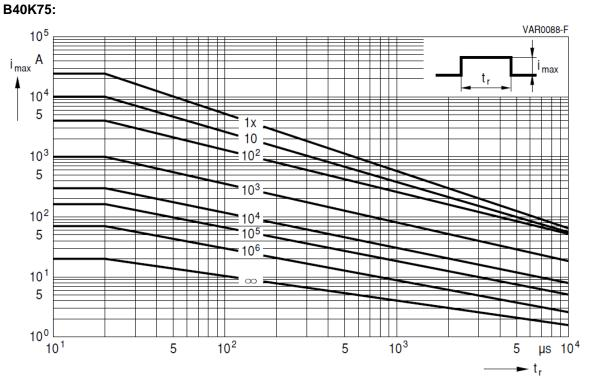
Reduction factor of maximum peak current for various numbers of pulses versus pulse duration.
