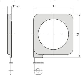
**Type C**: Customer specific \*QLK30 type with milled coating (not insulated):
