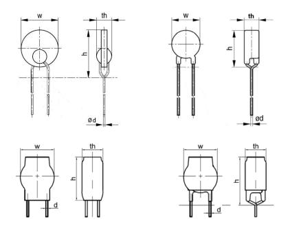
Data for the parameters  $w_{max}$ ,  $th_{max}$ ,  $h_{max}$  and Ød: See tables 1 and 2. The lead length is valid only for bulk packed components, for taped components IEC 60286-2 applies
