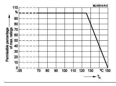
Maximum continuous a.c. or d.c. voltage with temperature.
