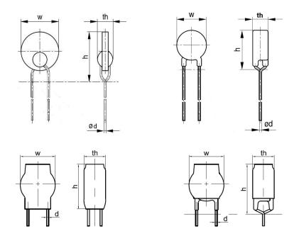
Data for the parameters  $w_{max}$ ,  $th_{max}$ ,  $h_{max}$  and Ød: See tables 1,2 and 3. The lead length is valid only for bulk packed components, for taped components IEC 60286-2 applies
